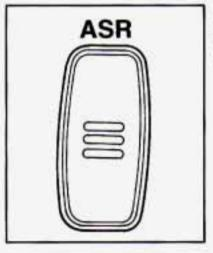
You can turn the system back on at any time by pressing the button again. The ASR OFF warning light should go off.
