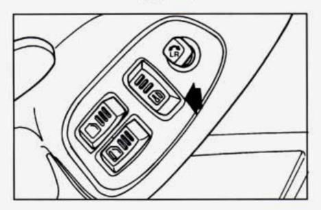
Push the power door lock switch to lock or unlock both doors at once.
