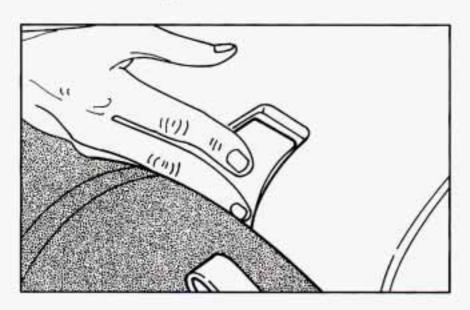
Open the trunk. Remove the middle piece of the cover by pushing in on the latch and lifting up on the cover.
