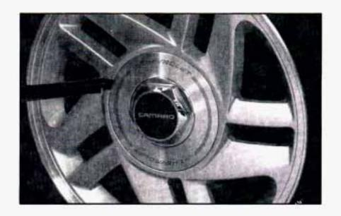
If your wheel has a center cap, pry it off using the wheel wrench.
