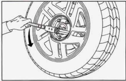
If your vehicle has optional alloy wheels, each wheel may have one locknut in place of the standard wheel nut. A special wheel lock key (removal tool) and instructions are located in the center console. Attach the wheel lock key to the socket of the wheel wrench. Remove the locking wheel nut by turning counterclockwise.
