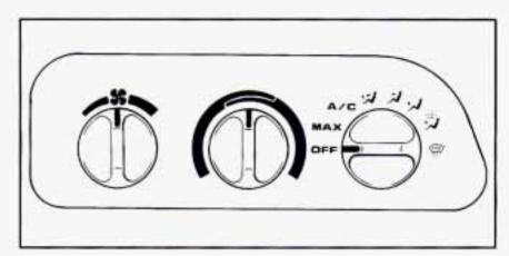
The air conditioning system uses the same controls as the heating system, except that the air control knob has two extra settings, described below. For an explanation of all the controls, see "Heater Controls" earlier in this section.
