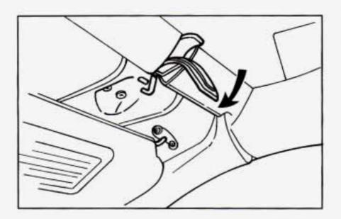
Pull down on the latches and align hooks with holes. Push forward on the larger part of the latch until it clicks. Do not force the latch. If it is hard to lock, the top is not properly aligned. If your vehicle suffers a power loss, such as a dead battery, you can still raise the top manually by rotating the valve in the left side of the trunk.
