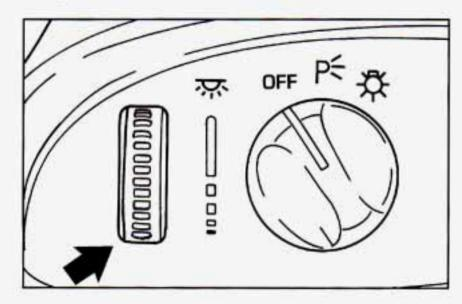
This switch controls the brightness of your instrument panel lights. Turn the switch to brighten or dim the lamps. If you turn the switch all the way up, your courtesy lamps will come on.
