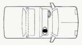
Your vehicle has a right front passenger air bag. Never put a rear-facing child restraint in this seat. Here's why:
