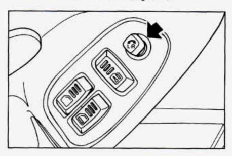
The electric mirror control is on the driver's door. To adjust either mirror, turn the switch to LEFT (L) or RIGHT (R). Then use the joystick to adjust the mirror.
