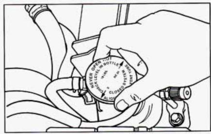
You can remove the radiator pressure cap when the cooling system, including the radiator pressure cap and upper radiator hose, is no longer hot. Turn the pressure cap slowly to the left until it first stops. (Don't press down while turning the pressure cap.)
