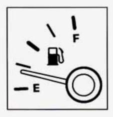
Your fuel gage shows about how much fuel is in your tank. The fuel gage works only when the ignition switch is in the RUN position. When the gage pointer first indicates EMPTY (E) you still have a little fuel left (about one to two gallons), but you need to get more right away.
