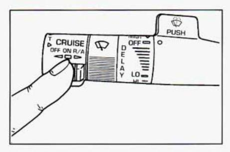
Suppose you set your cruise control at a desired speed and then you apply the brake or clutch pedal. This, of course, shuts off the cruise control. But you don't need to reset it. Once you're going about 25 mph (40 km/h) or more, you can move the cruise control switch from ON to R/A (Resume/Accelerate) for about half a second.
