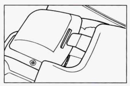
Remove the two side pieces of the boot cover by lifting the rear of cover and sliding them out of their slots.
