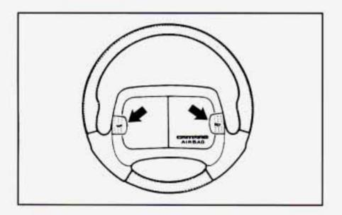
To sound the horn, press either horn symbol on your steering wheel.
