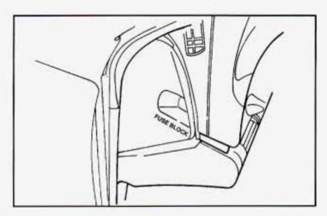
The wiring circuits in your vehicle are protected from short circuits by a combination of fuses, circuit breakers, and fusible thermal links in the wiring itself. This greatly reduces the chance of fires caused by electrical problems.
