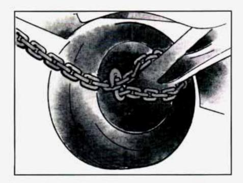
Attach a separate safety chain around outboard end of each lower control arm.
