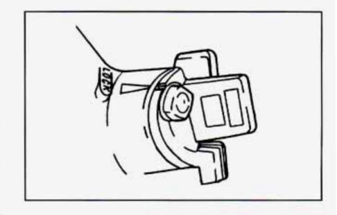
Key Release Button: If you have a manual transmission, your ignition lock has a key release button. You must press the button before you can take your key out of the ignition lock.
