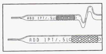
If the fluid level is in the acceptable range, push the dipstick back in all the way.
