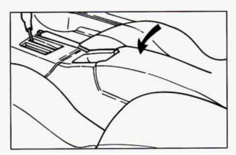
To use the storage area, pull up on the front end of the console. There is a cupholder and lamp and in the console.
