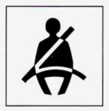
When the key is turned to RUN or START, a tone will come on for about eight seconds to remind people to fasten their safety belts, unless the driver's safety belt is already buckled. The safety belt light will also come on and stay on until the driver's belt is buckled.
