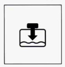
This red warning light should come on while you are starting your engine. If the light doesn't come on, have it repaired. The light also comes on when the coolant in your radiator is low. You may need to add coolant. See the Index under "Engine Coolant."
