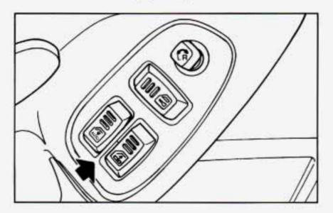
With power windows, switches on the door control each window when the ignition is on or when RAP is present. (See "Retained Accessory Power" in the Index.)
