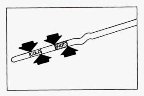
The fluid level must be in the COLD area for a cold check or in the HOT area or cross-hatched area for a hot check
