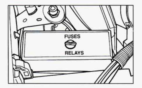
The other is in the engine compartment. Open the cover on either of the boxes to expose the fuses.
