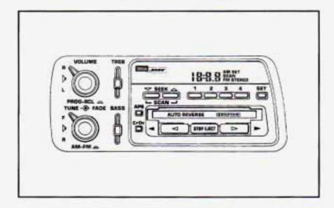
SCAN: The scan function uses the same two buttons as the seek function. To go to the next higher station and stay there for a few seconds, press and hold SEEK ▲ and then press SEEK ▼ for an instant.
