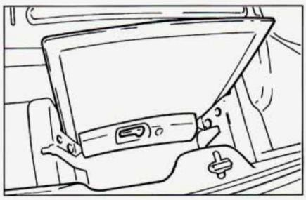
Open the close-out panel completely. Place the panel in the correct slot (driver or passenger) in the rear area of your vehicle. Make sure the handle is open and facing you when you put it in the storage slot.
