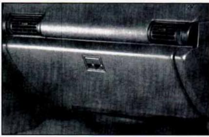
To open the glove box, lift up on the lever. Use your door key to lock and unlock it. The glove box has a light inside.
