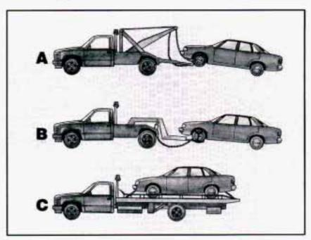
Try to have a GM dealer or a professional towing service tow your Chevrolet. The usual towing equipment is a sling-type (A) or a wheel-lift (B) or car carrier (C) tow truck. If your vehicle has been changed or modified since it was factory-new by adding aftermarket items like fog lamps, aero skirting, or special tires and wheels, these instructions and illustrations may not be correct.
