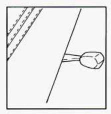
Move the lever under the passenger's front seat to unlock it.
