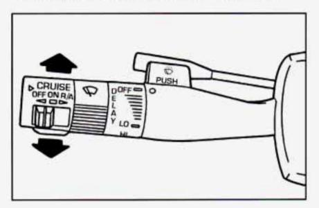
The turn signal has two upward (for Right) and two downward (for Left) positions. These positions allow you to signal a turn or a lane change.
