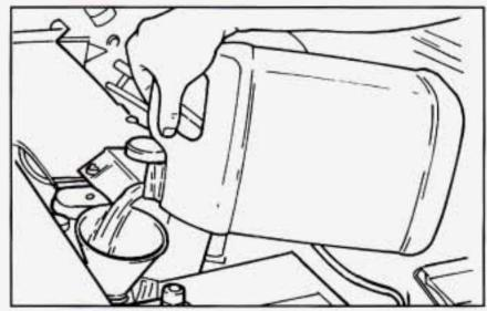
Then fill the coolant recovery tank to the proper level.
