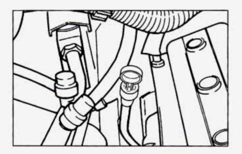
Turn off the engine and give the oil a few minutes to drain back into the oil pan. If you don't, the oil dipstick might not show the actual level.
