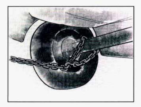
Attach a separate safety chain around each outboard end of the rear axle.
