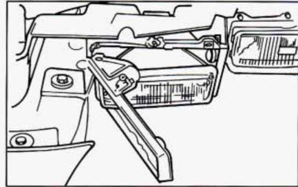
Remove the Torx<sup>®</sup> head screws at the end of the aiming ring.  The aiming ring will swing open like a gate. Remove the aiming ring from the assembly. Place it face down, with the aim indicator up. Be careful not to damage the aiming bubble.
