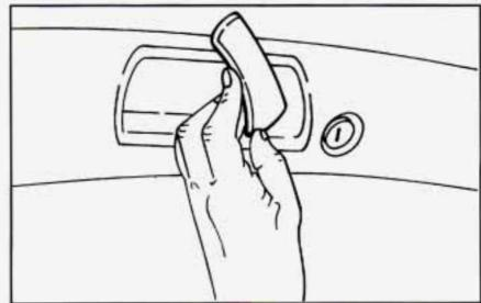
The door key unlocks the panels. Turn the key to the left to unlock the panel.
