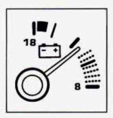
You can read battery voltage on your voltmeter. If it reads less than 11 volts or more than 16 volts while your engine is running, and it stays there, you may have a problem with the electrical charging system. Have it checked right away. Driving with the voltmeter reading in a warning zone could drain your battery.
