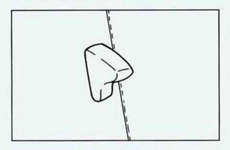
The front seatbacks fold forward to let people get into the back seat. To fold a seatback forward, push the seatback toward the rear as you lift the latch located on the lower backside of the seatback. Then the seatback will fold forward. When you return the seatback to its original position, make sure the seatback is locked. The latch must be down for the seat to work properly.
