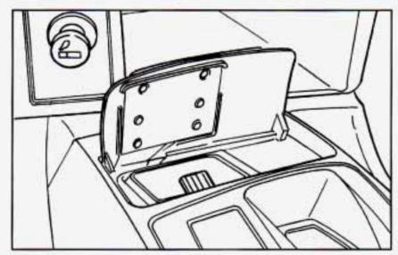
Lift up the cover to open the ashtray. To remove it, lift up on the right side of the ashtray. If you have an automatic transmission, the ashtray is near the front of your console. If you have a manual transmission, the ashtray is near your cupholder.
