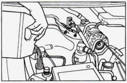
Fill the radiator with the proper mix, up to the base of the filler neck.
